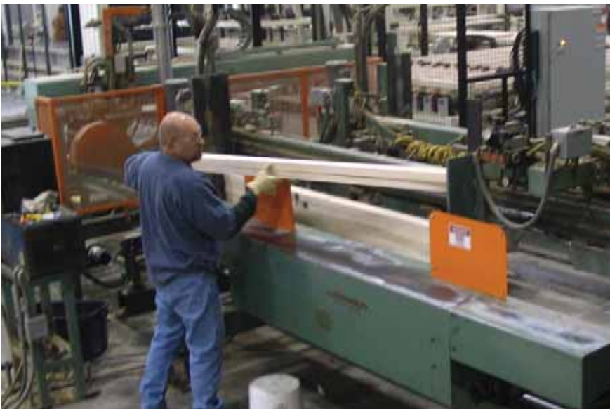
Operator Al Gronau loads a stile cartridge on Lexington Brainerd's new automated door core banding line.
