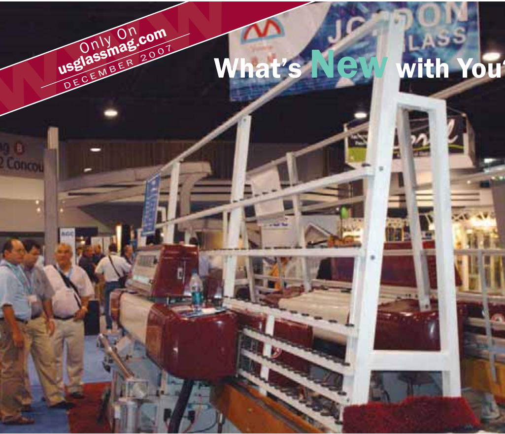
The 9-spindle DJ252D machine for shower enclosure fabrication was one of several machines on display from Jordan Glass.
