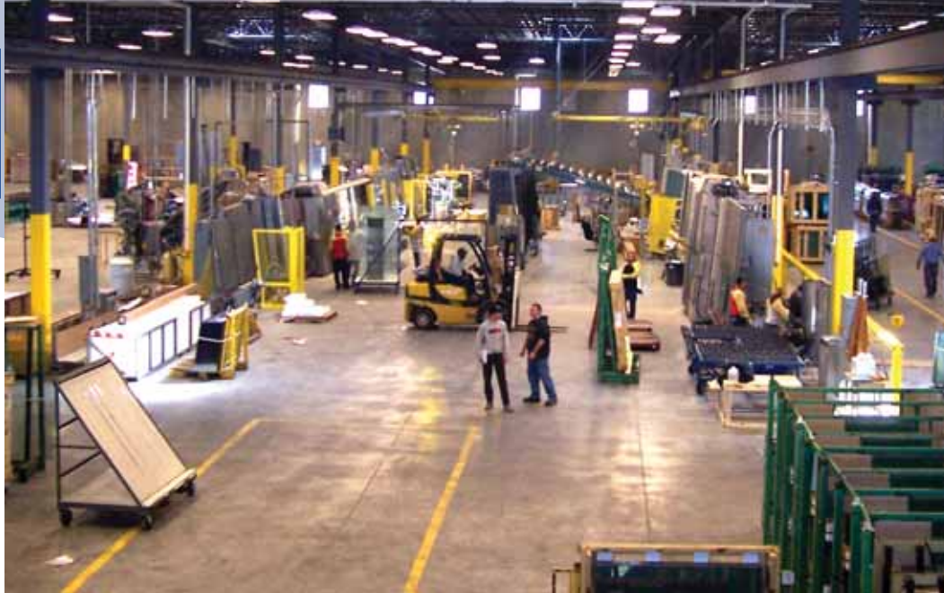
JEB's new plant is 200,000 square feet and has three IG lines, three tempering lines and one laminating line.
