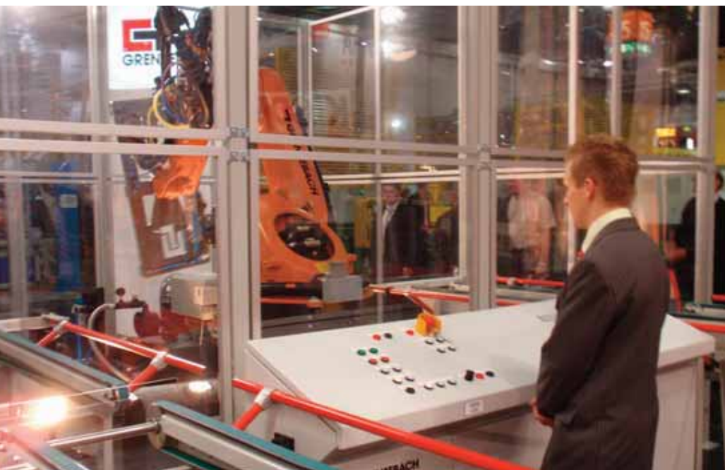
Grenzebach's new equipment can seam and grind edges of architectural or solar glass.
