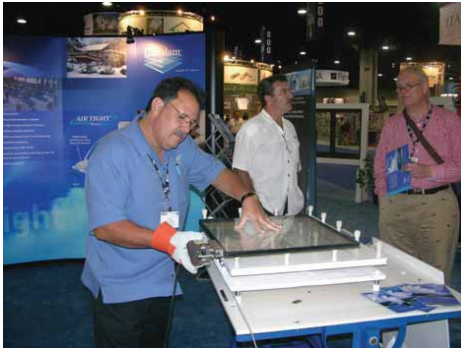
Glaslam demonstrated the process of making IGUs with its new SmartEdge warm-edge spacer.
